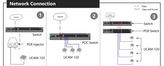
Connect devices based on site situation and quantity of devices using either of three optional networking structures.
